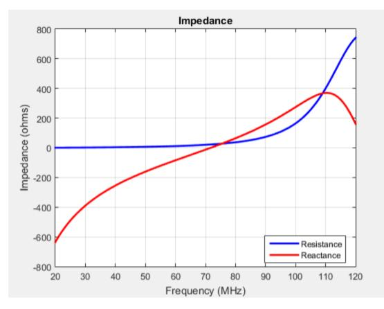
You can observe the first resonance is at approximately 71 MHz. To lower the resonance frequency, recalculate the height of the monopole to quarter wavelength. The frequency of operation is also lower. You must also have to increase the size of the corresponding ground plane. This increase in size means that to achieve similar performance at a lower frequency, you need a larger antenna. This approach is not possible due to physical space constraints.
