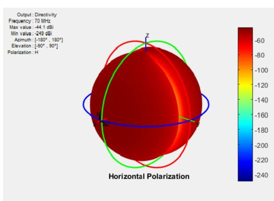
d = dipole; pattern(d,70e6,'Polarization','H')
