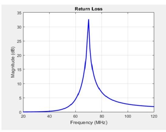
Return loss plots also give the operating bandwidth of the antenna. Antenna bandwidth is the frequency band over which the magnitude of return loss is greater than 10 dB. Use the returnLoss function to calculate the return loss of any antenna in the Antenna Toolbox library.
