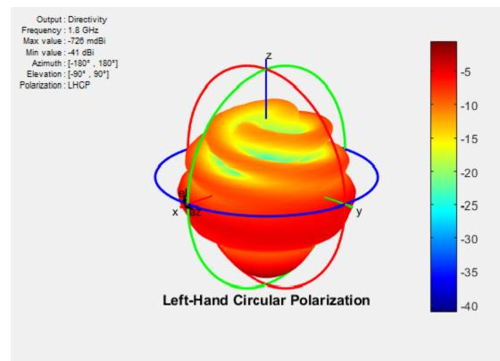
For efficient communications, the antennas at the transmitting and receiving end must have same polarization.
