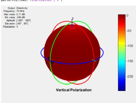
d = dipole; pattern(d,70e6,'Polarization','V')
